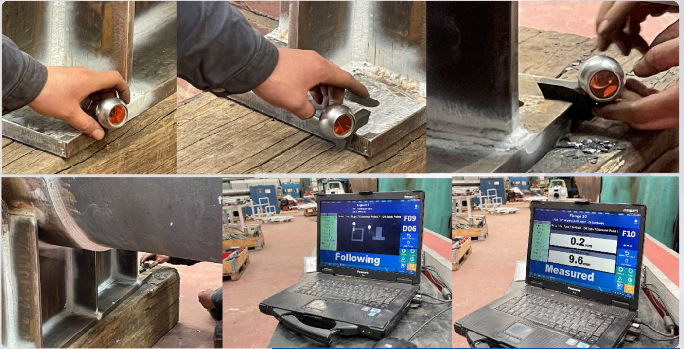
SUPPORT BASE-PLATE LOCATION AND FLATNESS CHECKS.
